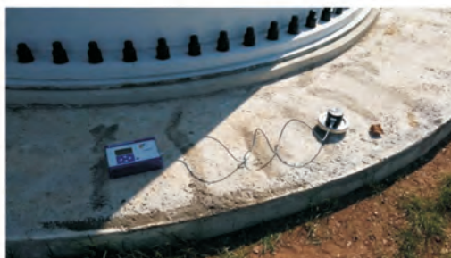
Figure 5 – Fixing a vibration indicator on WPU foundation
