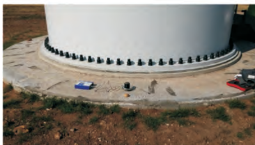
Figure 5 – Fixing a vibration indicator on WPU foundation
