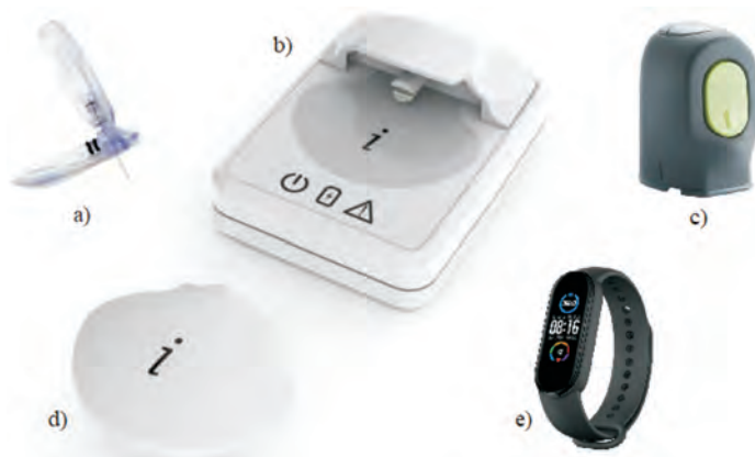
Figure 4 – a) Enlite MMT-7008A; b) Docking station; c) Enlite MMT-7510; d) iPro2 MMT-7745WW; e) Xiaomi Mi Band 5
