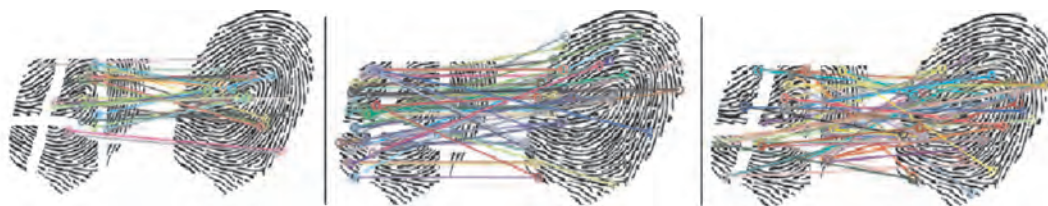
Figure 2 – Evaluation of 30 keypoint descriptors ORB (left), SIFT (center), SURF (right)
