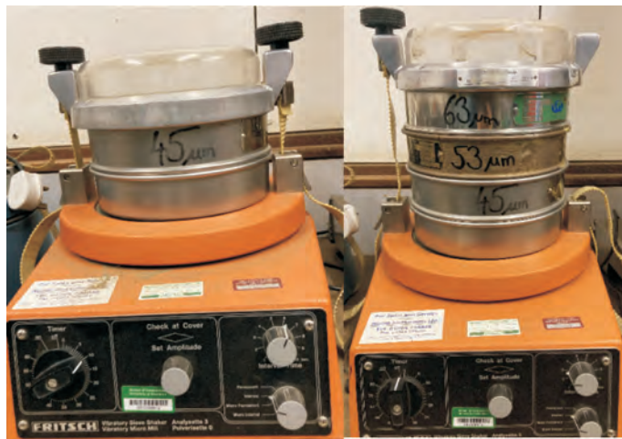
Figure 1 – Sieving of crushed rock samples on vibratory sieve shaker
