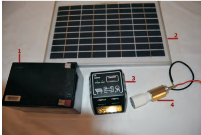
Figure 3 – Standalone power supply unit: 1 – rechargeable battery (MHB); 2 – solar panel; 3 – charge controller for the solar panel; 4 – car charger providing 5V current
