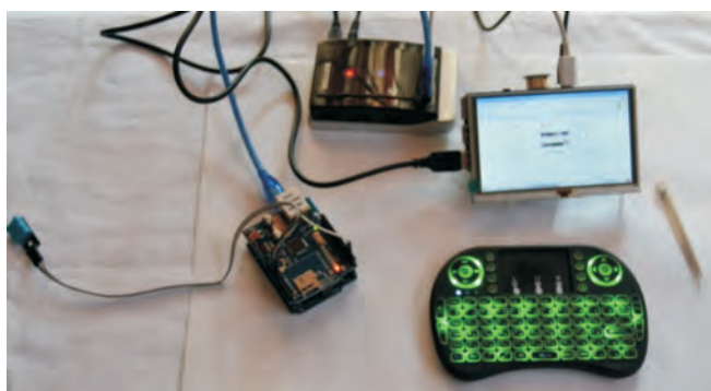
Figure 6 – Receiving temperature and humidity data on the screen
