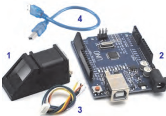
1 – FPM10A optical fingerprint scanner; 2 – Arduino UNO; 3 – wires to connect the scanner to the Arduino; 4 – USB cable for Arduino
