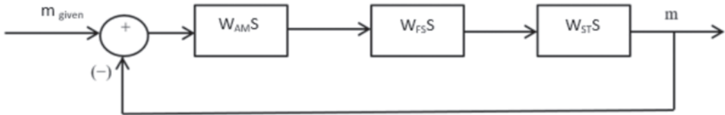
Figure 3 – Block diagram of the linearized contour of the control object
